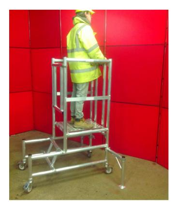
Dimensions — Platform at 1M x Width –0.65M x Depth 1.3M
