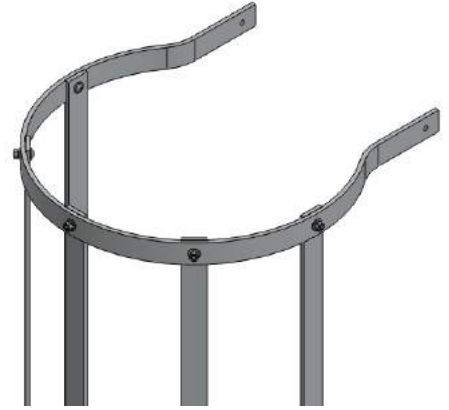
2: Fit remaining strap to upper hoop Use M10 x 35 bolt with dome head facing inwards
