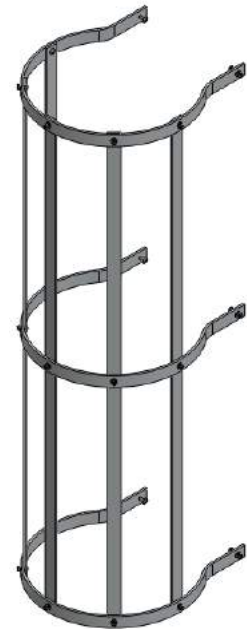
4: Complete Cage Ensure all bolts are fully tightened and all washers are in place the cage is now complete
