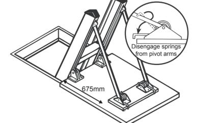
Note: The ladder can now be used safely for access into the loft to complete the installation.
