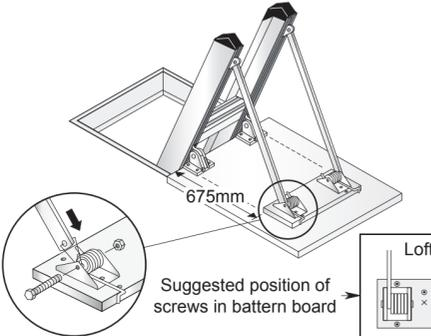
Suggested position of screws in batten board
