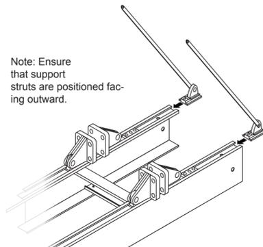
Note: Ensure that support struts are positioned facing outward.
