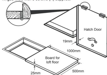
The Twist Catch Assembly and Pull Brackets should be fitted as shown.
